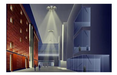
In the vast entrance atrium we washed the rear façade of the Granary Building to emphasise the warmth and texture of the brick, using a custom linear system designed to mimic the original door rails. Opposing this, we softly washed the large expanses of white plaster walls and soffit of the south façade of the new building.
